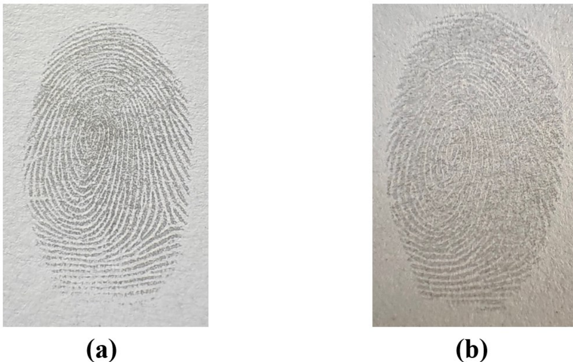
Figure 4. (a) Developed latent fingerprints on a white porous paper by using NCO nanoparticles. (b) Developed latent fingerprints on a white porous paper by using commercial black magnetic powder.
